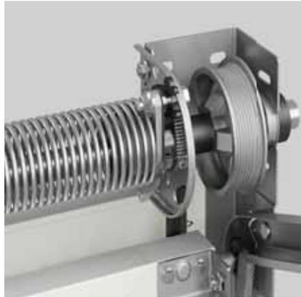
Torsion springs are equipped with **spring breaks** that stop the door leaf from falling in the case of spring breakage. This protection system is supplied at no extra cost to ensure safe operation.
